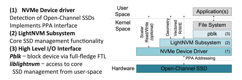
With LightNVM, a system in user space can fully control data placement and I/O scheduling across multiple openchannel SSDs
