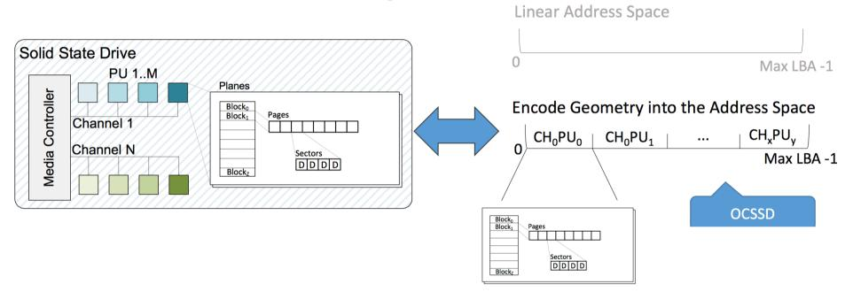
PPA provides (i) a hierarchical address space, based on SSD intrinsic parallelism (channels and PUs) and media characteristics, and (ii) vectored I/Os.
