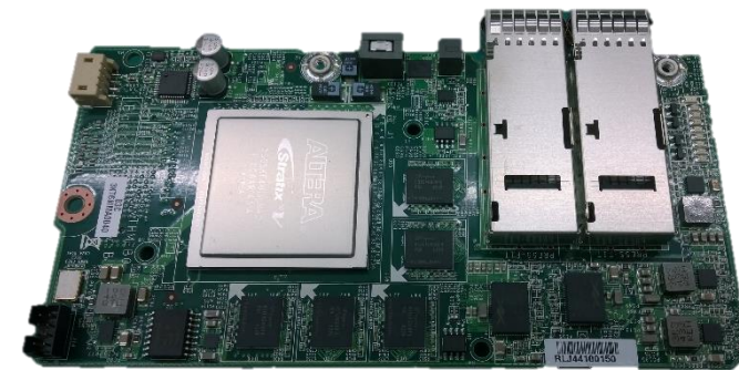
WCS Gen4.1 Blade with Mellanox NIC and Catapult FPGA
